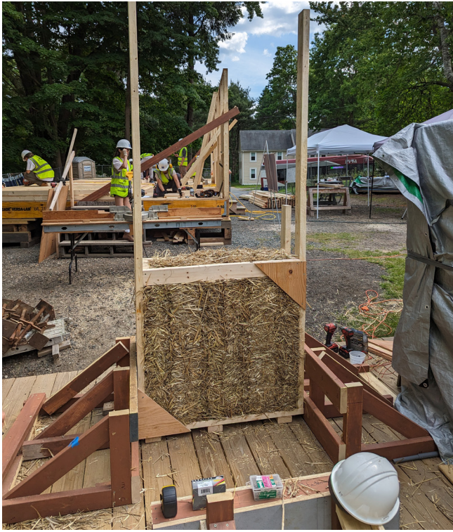
Figure 8. Straw bale compression assembly. Photo by Josey Wermuth.
